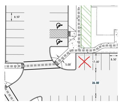
In the diagram shown above, (at least) the two parking stalls shown crossed out will be reduced in depth to 17-ft. This is allowed pursuant to BDC Section 60.30.15 (Note 6). However, BDC Section 60.55.25.10.B.5 states that:
